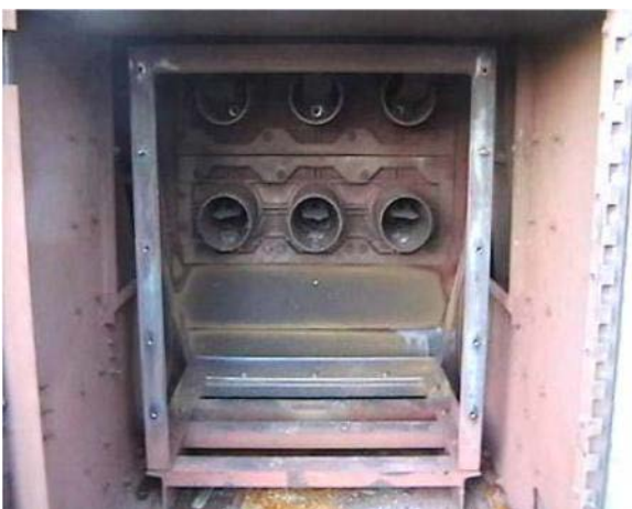
Test result with 500ms arcing time
